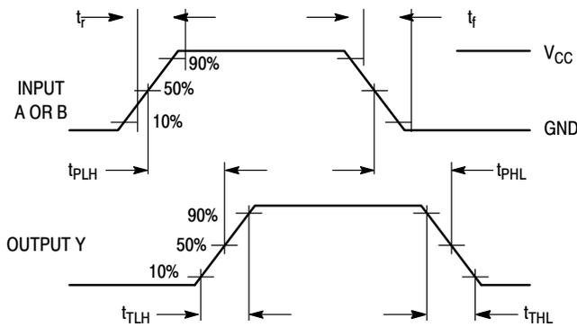
Figure 1. Switching Waveforms
