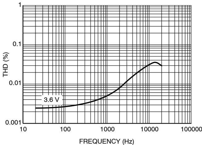
**Figure 7. Total Harmonic Distortion Plus Noise Versus Frequency**
