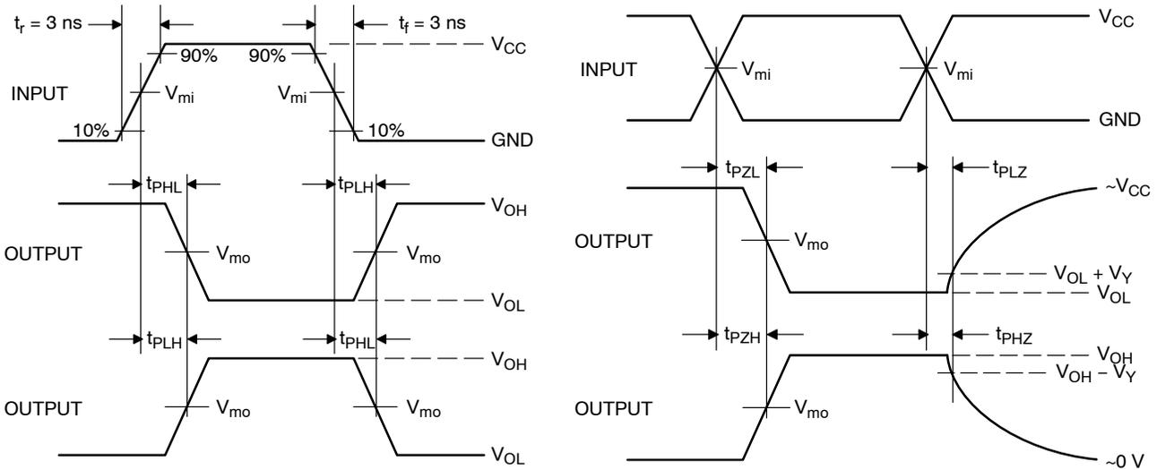
**Figure 11. Switching Waveforms**
