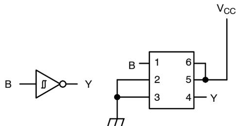
Figure 9. Inverter (When A = "L" and C = "H")
