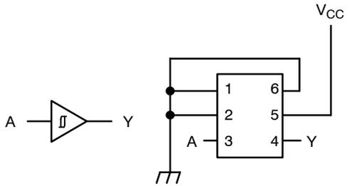
Figure 8. Buffer (When B = C = "L")
