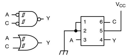
Figure 6. 2-Input OR (When B = "L")
