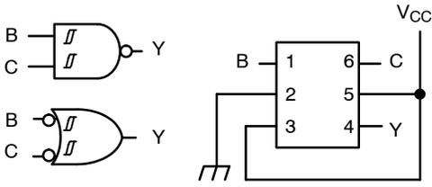
Figure 3. 2-Input NAND (When A = "H")
