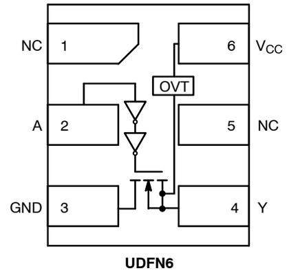
Figure 2. Pinout (Top View)
