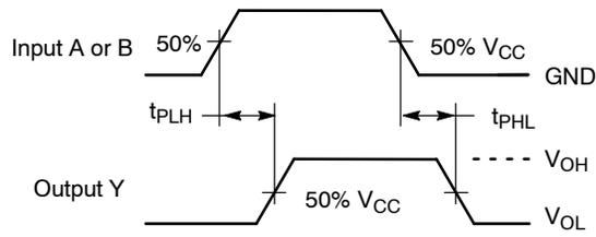
**Figure 4. Switching Waveforms**
