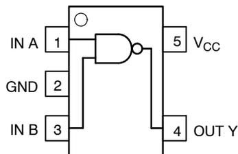
Figure 1. Pinout
