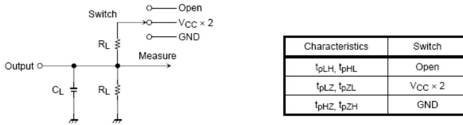
Figure 5. Test Circuit
