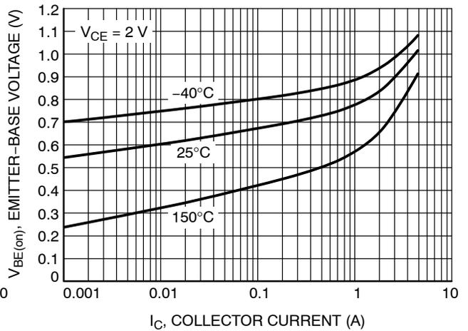
Figure 7.  $V_{BE(on)}$  Voltage
