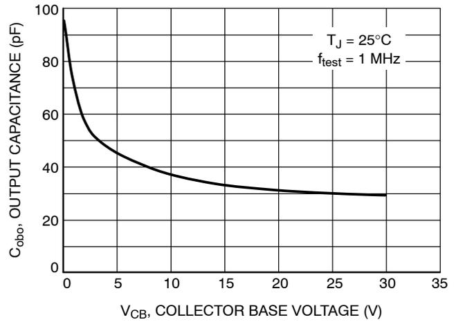
Figure 11. Output Capacitance
