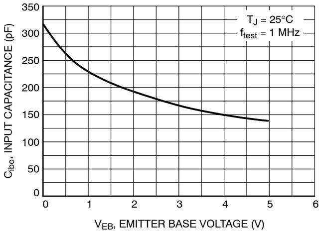
Figure 10. Input Capacitance
