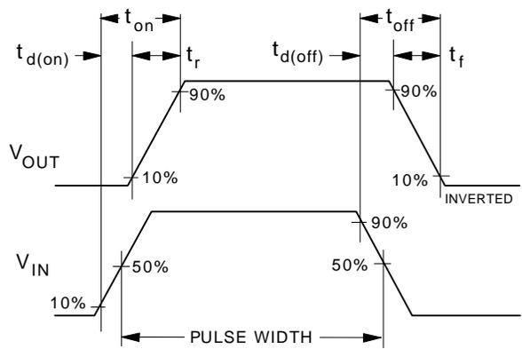
Figure 12. Switching Waveforms.
