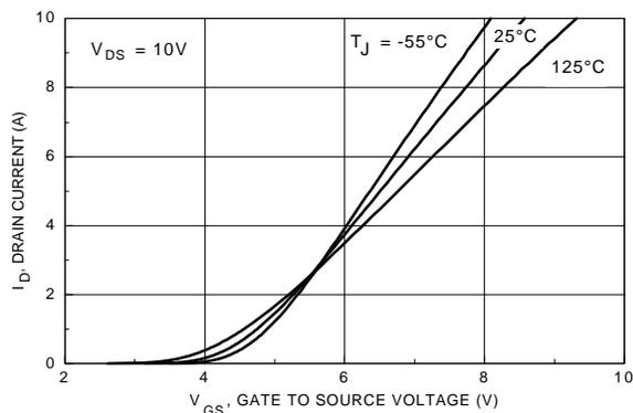
Figure 5. Transfer Characteristics.
