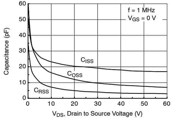
Figure 8. Capacitance Characteristics
