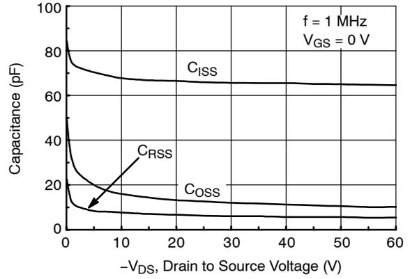
Figure 19. Capacitance Characteristics
