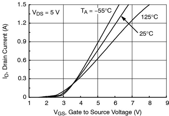
Figure 5. Transfer Characteristics
