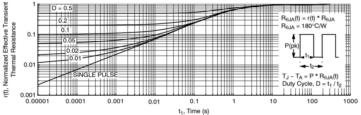
Figure 22. Transient Thermal Response Curve
