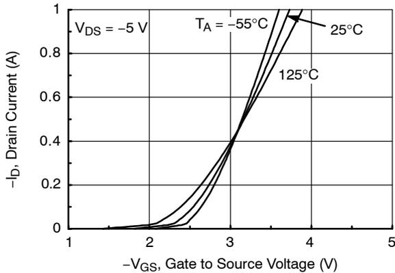
Figure 16. Transfer Characteristics
