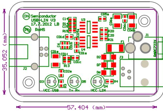
Figure 9. LIN Interface V3 Top Assembly Drawing
