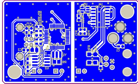
Figure 12. LIN Interface V3 PCB Bottom Composite Drawing
