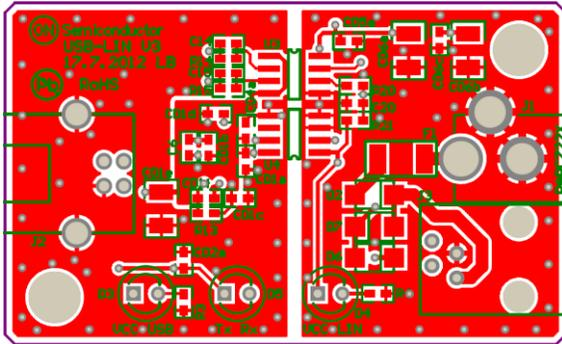
Figure 11. LIN Interface V3 PCB Top Composite Drawing
