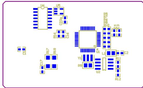
Figure 10. LIN Interface V3 Bottom Assembly Drawing
