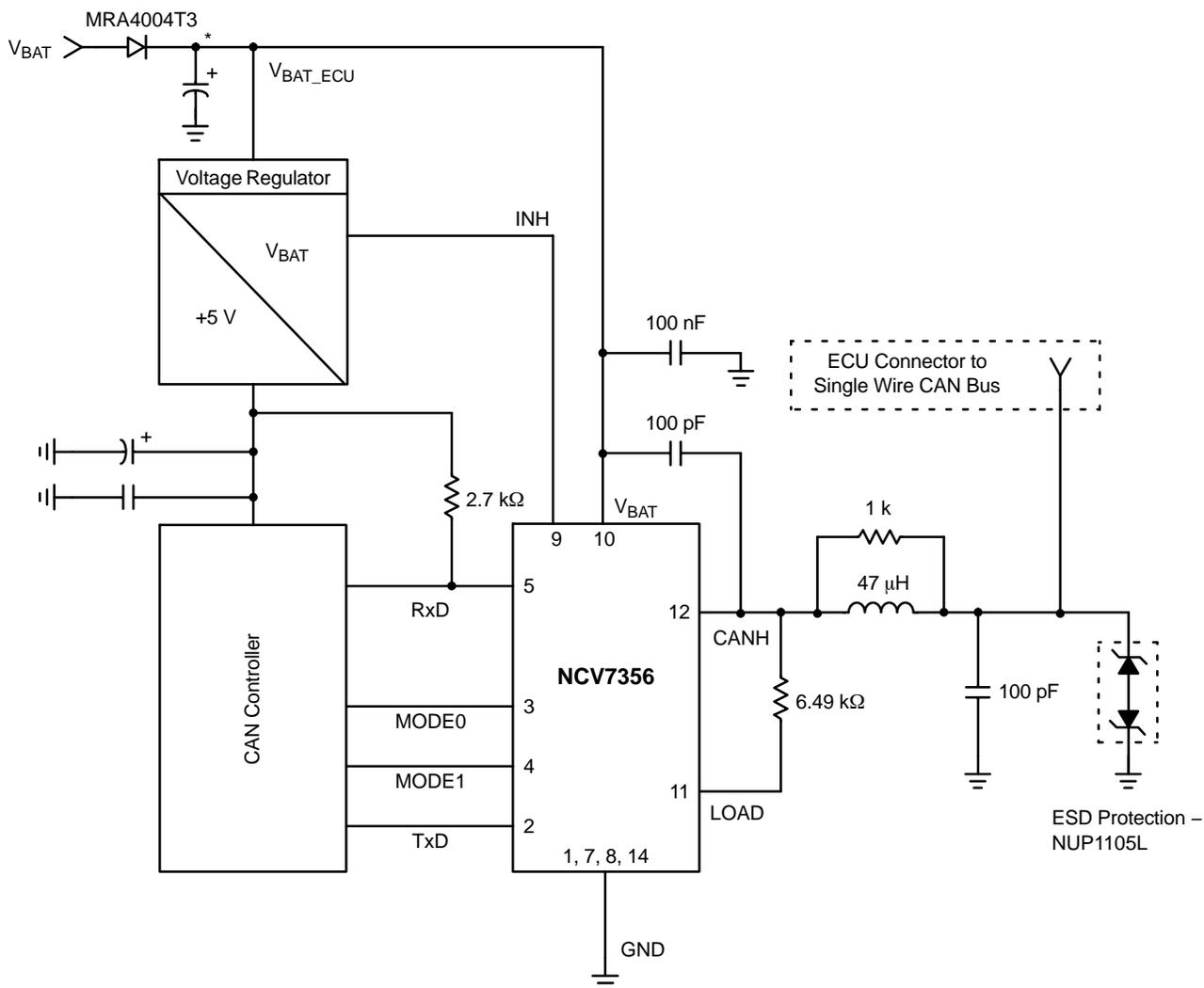
\*Recommended capacitance at V<sub>BAT\_ECU</sub> > 1.0 μF (immunity to ISO7637/1 test pulses)
