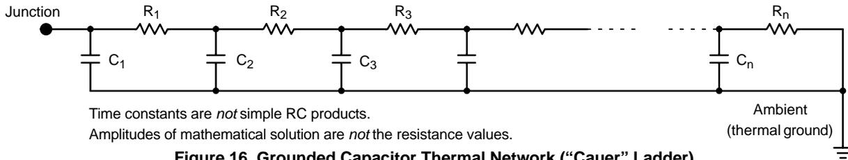
**Figure 16. Grounded Capacitor Thermal Network (“Cauer” Ladder)**
