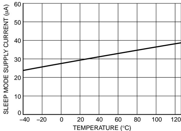
**Figure 5. Sleep Mode Supply Current vs. Temperature**
