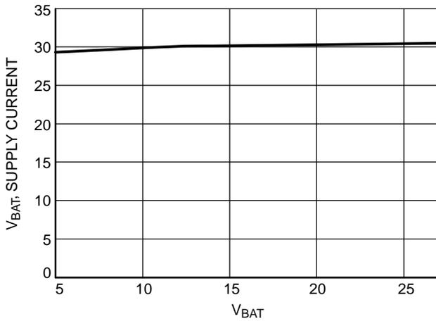
**Figure 3. Normal Mode Supply Current Dominant vs.  $V_{BAT}$**
