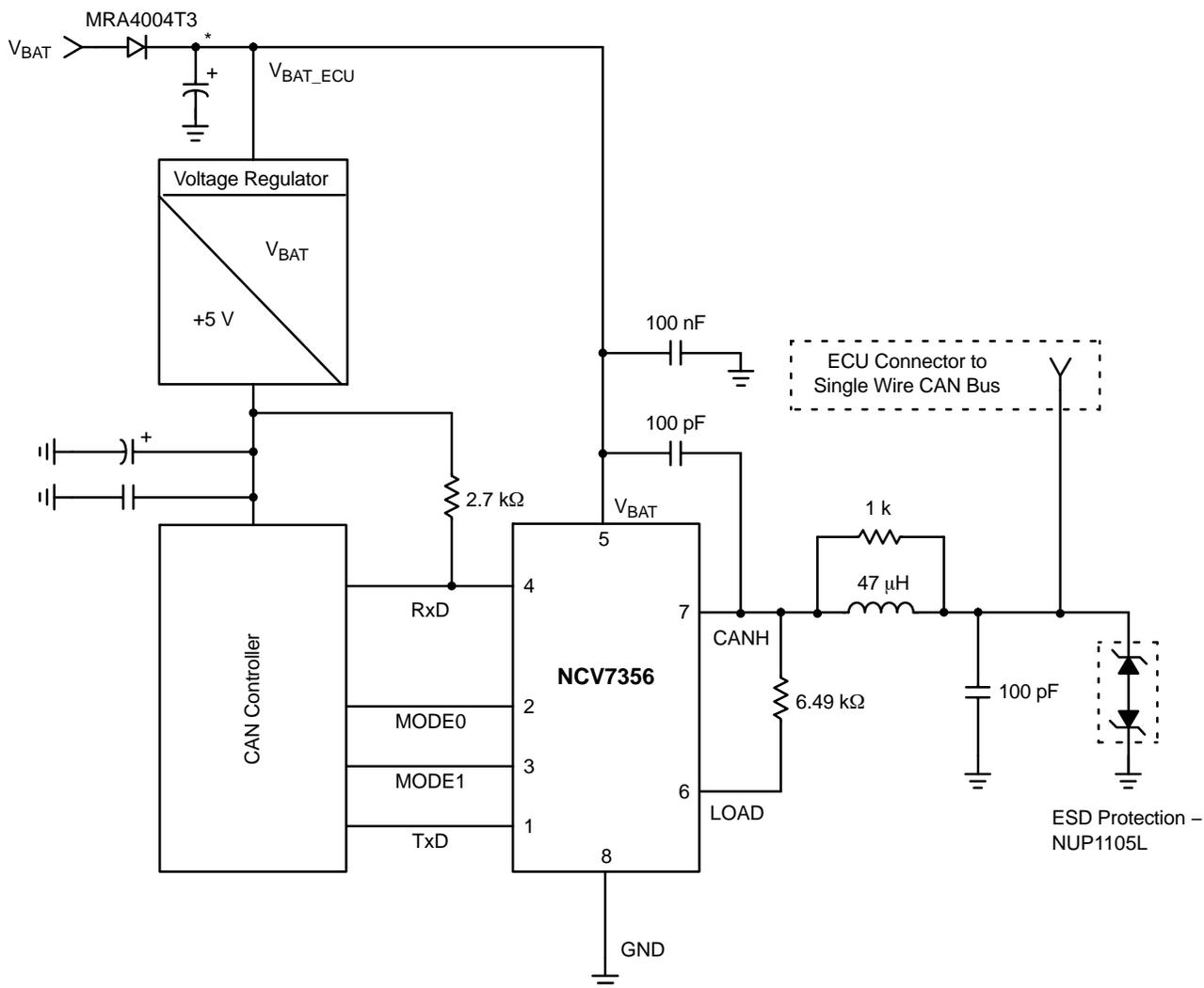
\*Recommended capacitance at  $V_{BAT\_ECU} > 1.0 \mu F$  (immunity to ISO7637/1 test pulses)
