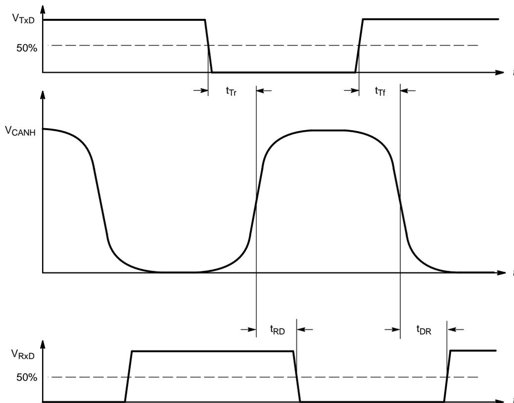
Figure 6. Input/Output Timing
