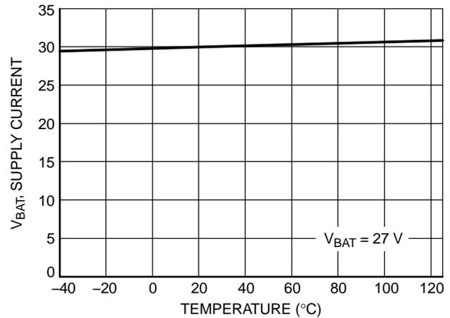
**Figure 4. Normal Mode Supply Current Dominant vs. Temperature**
