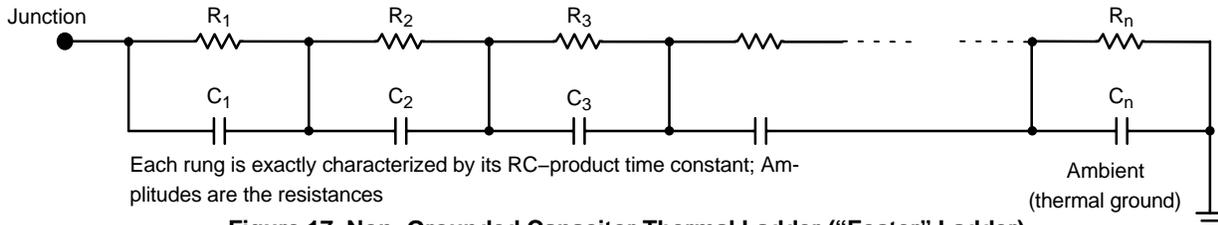
**Figure 17. Non-Grounded Capacitor Thermal Ladder (“Foster” Ladder)**
