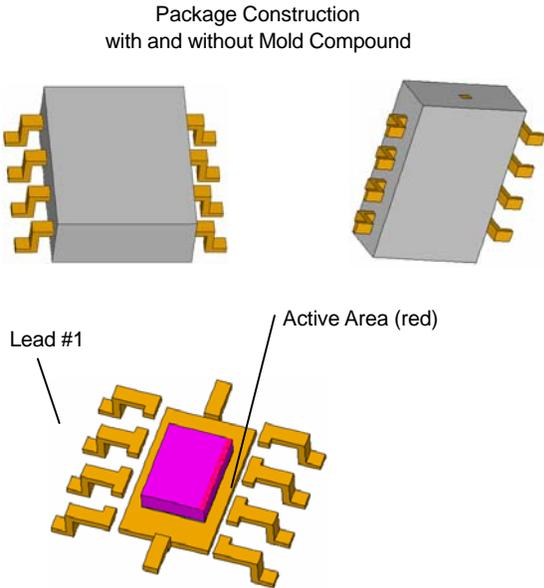
Figure 13. Internal construction of the package simulation.
