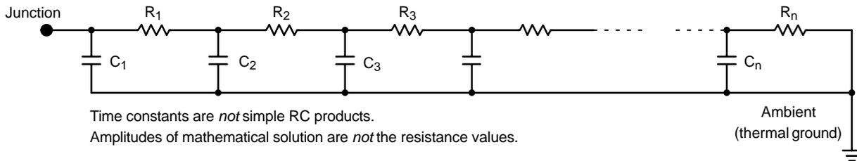
Figure 23. Grounded Capacitor Thermal Network ("Cauer" Ladder)
