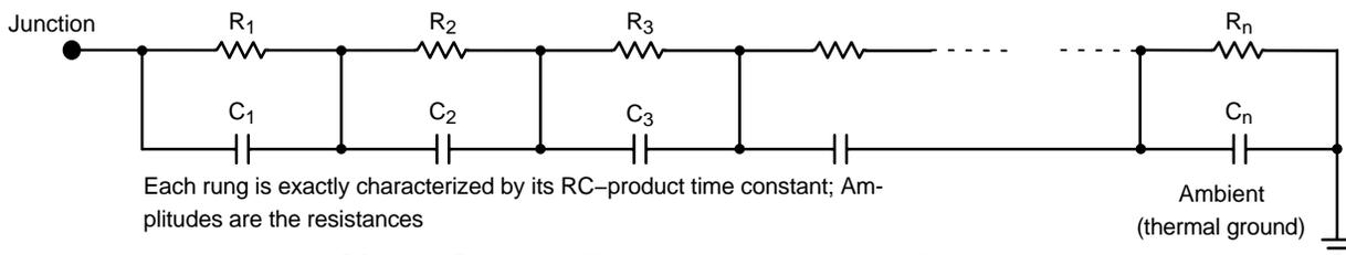
Figure 24. Non-Grounded Capacitor Thermal Ladder ("Foster" Ladder)
