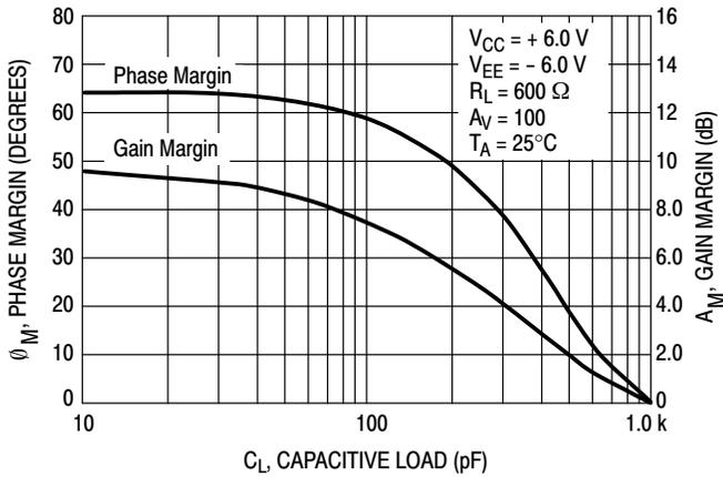
Figure 22. Gain and Phase Margin versus Capacitive Load
