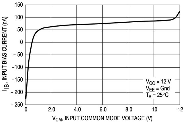
Figure 6. Input Bias Current versus Common Mode Voltage
