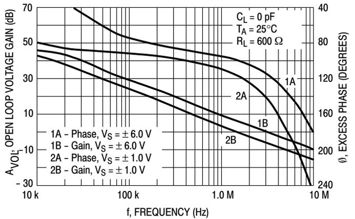
Figure 19. Voltage Gain and Phase versus Frequency
