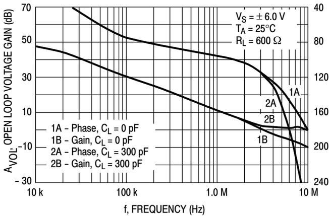
Figure 18. Voltage Gain and Phase versus Frequency
