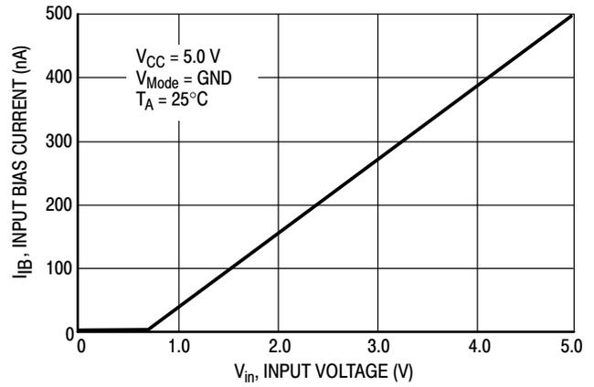
Figure 3. Comparator Input Bias Current versus Input Voltage
