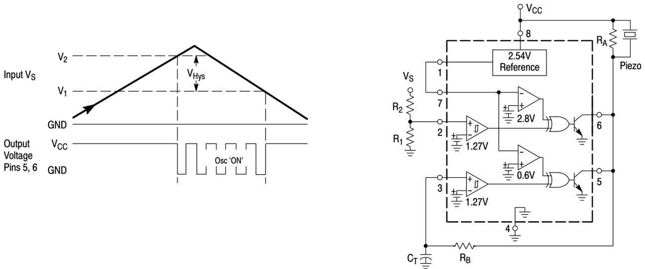
The above figure shows the MC34161 configured as an overvoltage detector with an audio alarm. Channel 1 monitors input voltage  $V_S$  while channel 2 is connected as a simple RC oscillator. As the input voltage increases from ground, the output of channel 1 allows the oscillator to turn 'ON' when  $V_S$  exceeds  $V_2$ .
