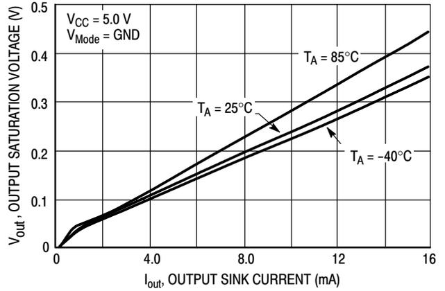
Figure 11. Output Saturation Voltage versus Output Sink Current
