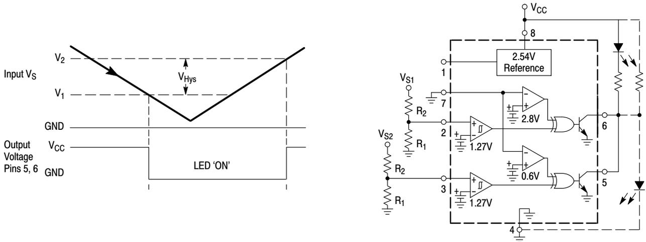
The above figure shows the MC34161 configured as a dual positive undervoltage detector. As the input voltage decreases towards ground, the LED will turn 'ON' when  $V_{S1}$  or  $V_{S2}$  falls below  $V_1$ . With the dashed line output connection, the circuit becomes a dual positive overvoltage detector. As the input voltage increases from ground, the LED will turn 'ON' when  $V_{S1}$  or  $V_{S2}$  exceeds  $V_2$ .
