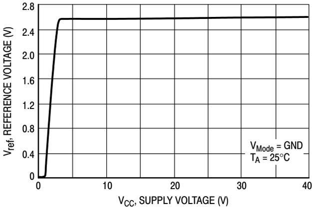
Figure 8. Reference Voltage versus Supply Voltage
