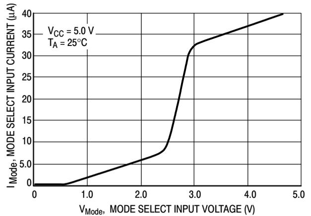
Figure 7. Mode Select Input Current versus Input Voltage
