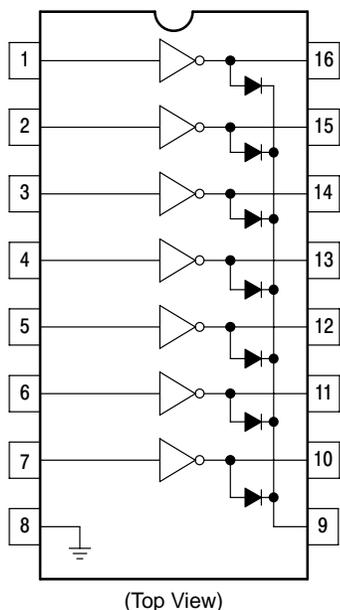
Figure 2. PIN CONNECTIONS
