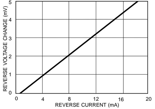
Figure 4. Change in Reverse Voltage vs. Reverse Current
