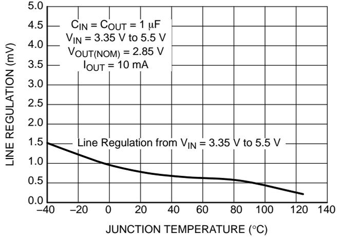
Figure 33. Line Regulation vs. Temperature
