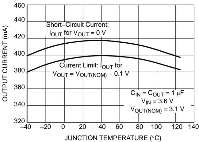
**Figure 28. Short-Circuit Limit vs. Temperature**
