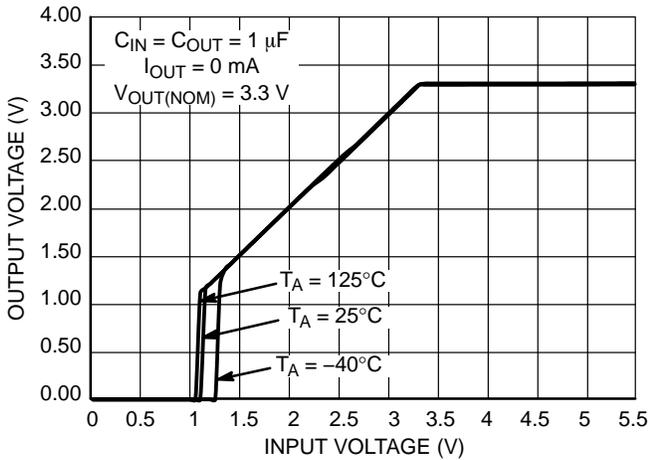
**Figure 16. Output Voltage vs. Input Voltage**
