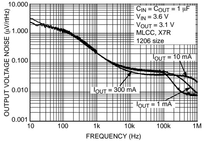
Figure 49. Output Noise Density vs. Frequency
