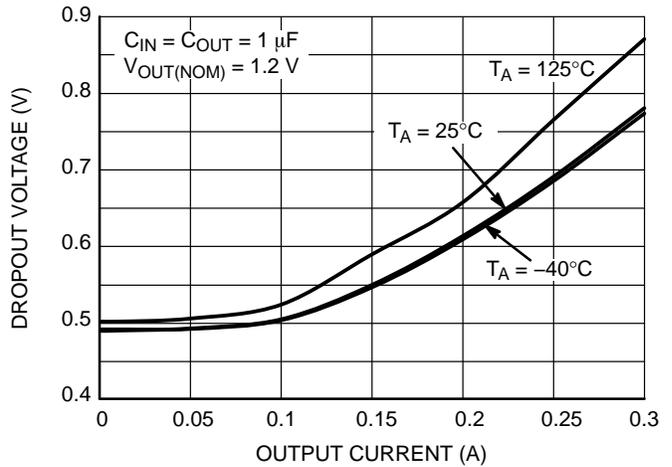
**Figure 17. Dropout Voltage vs. Output Current**
