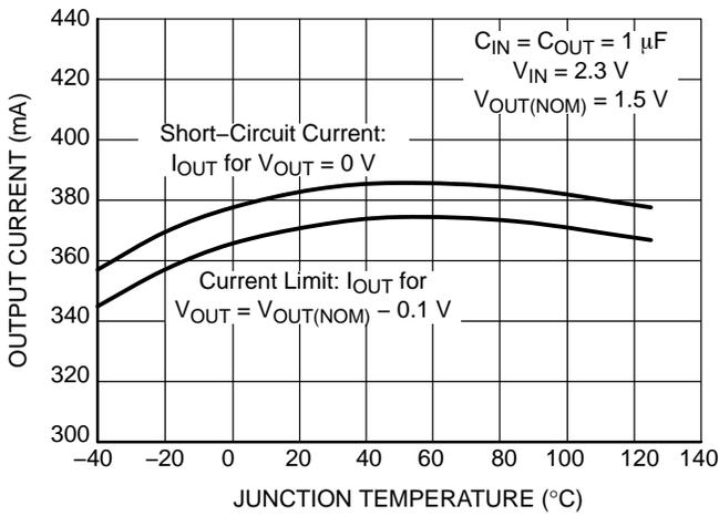
**Figure 24. Short-Circuit Limit vs. Temperature**
