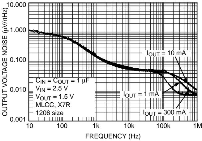
Figure 48. Output Noise Density vs. Frequency
