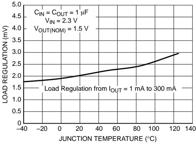
**Figure 38. Load Regulation vs. Temperature**
