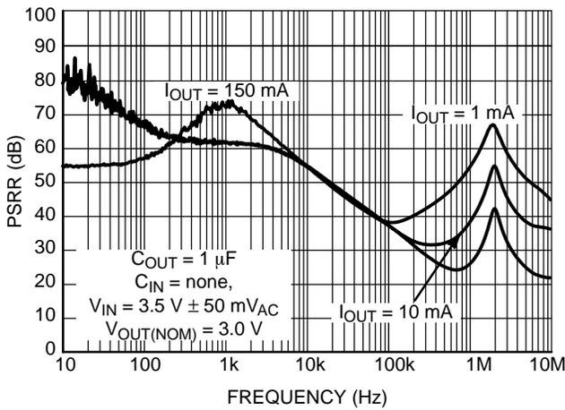
Figure 46. PSRR vs. Frequency
