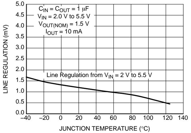
Figure 31. Line Regulation vs. Temperature
