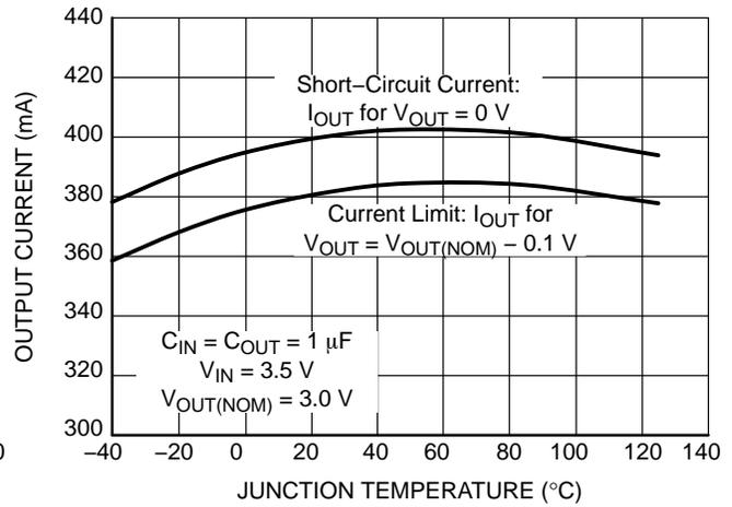
**Figure 27. Short-Circuit Limit vs. Temperature**
