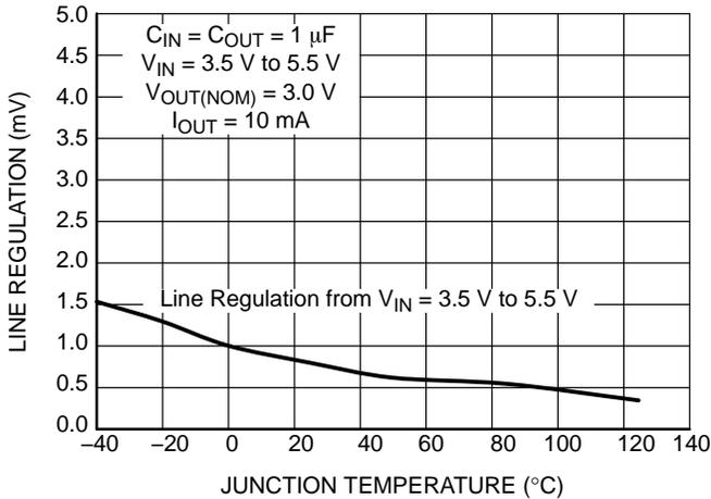
Figure 34. Line Regulation vs. Temperature
