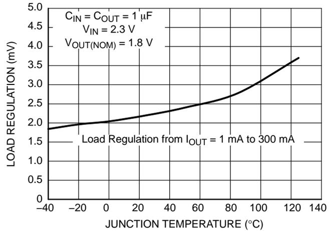
**Figure 39. Load Regulation vs. Temperature**
