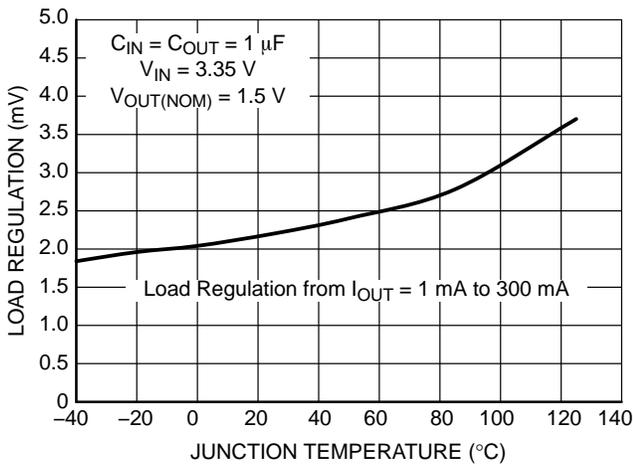
**Figure 40. Load Regulation vs. Temperature**
