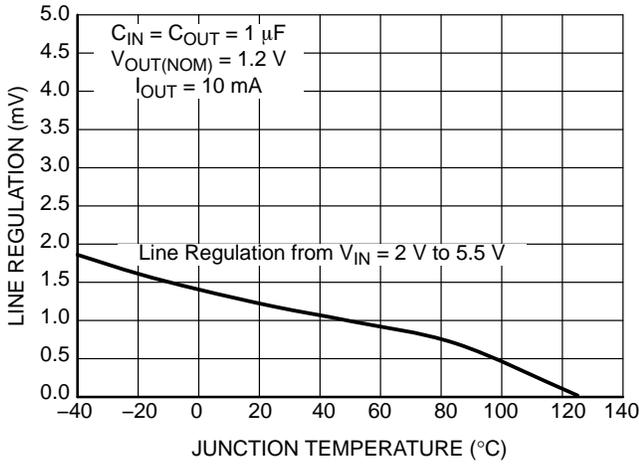
Figure 30. Line Regulation vs. Temperature
