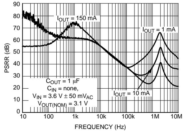
Figure 47. PSRR vs. Frequency
