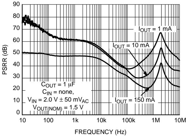
Figure 44. PSRR vs. Frequency
