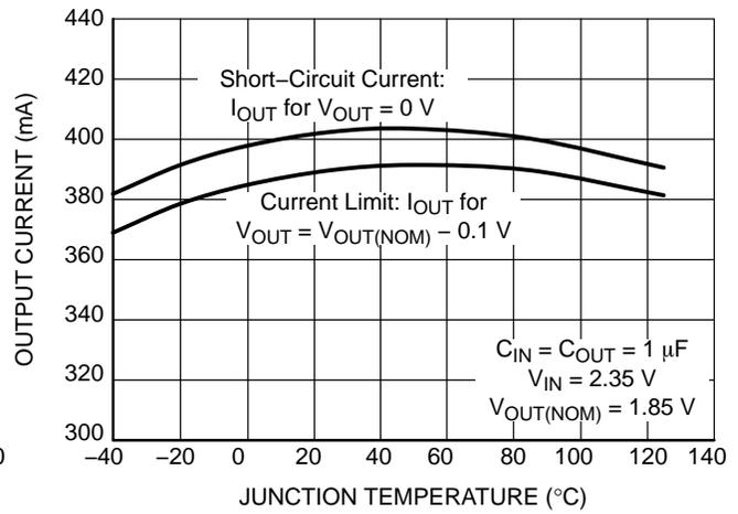
**Figure 25. Short-Circuit Limit vs. Temperature**
