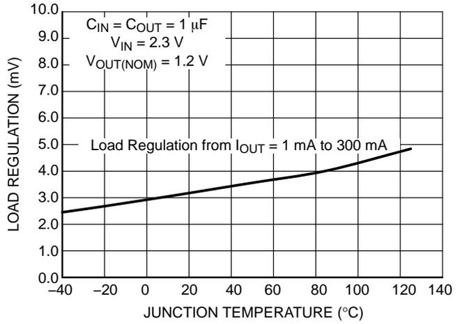
**Figure 37. Load Regulation vs. Temperature**
