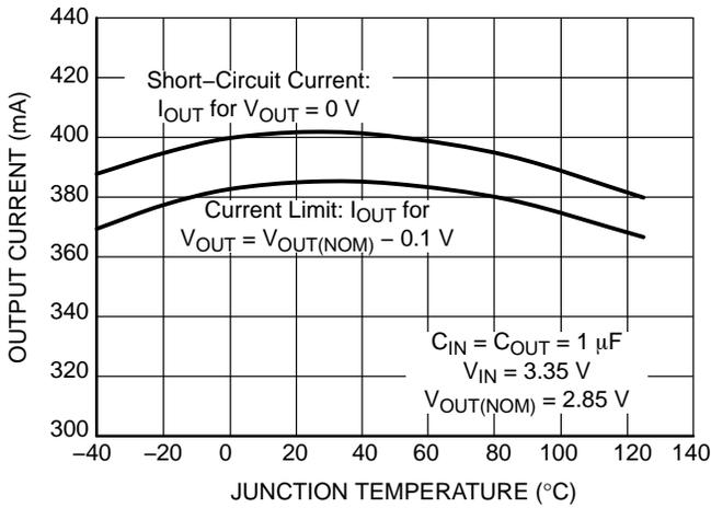
**Figure 26. Short-Circuit Limit vs. Temperature**
