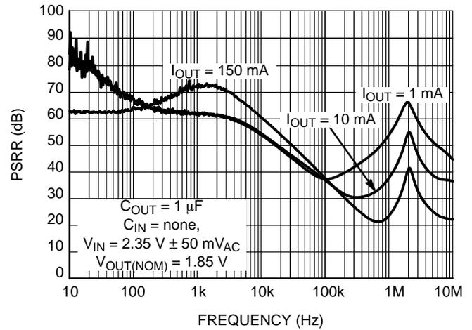
Figure 45. PSRR vs. Frequency
