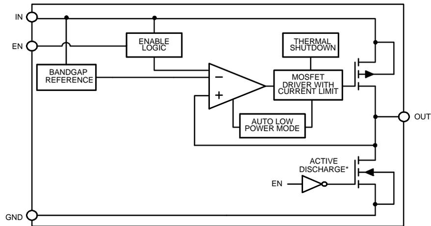
\*Active output discharge function is present only in NCP717AMXyyyTCG and NCP717CMXyyyTCG devices. yyy denotes the particular  $V_{OUT}$  option.
