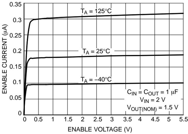
Figure 50. Enable Input Current vs. Enable Voltage
