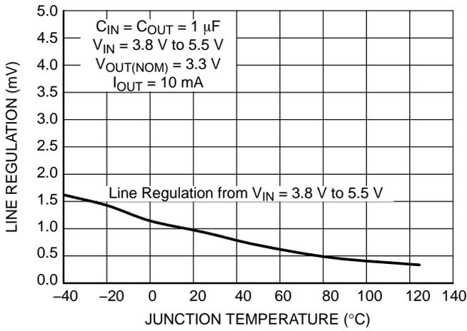
**Figure 36. Line Regulation vs. Temperature**
