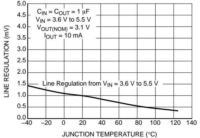
Figure 35. Line Regulation vs. Temperature
