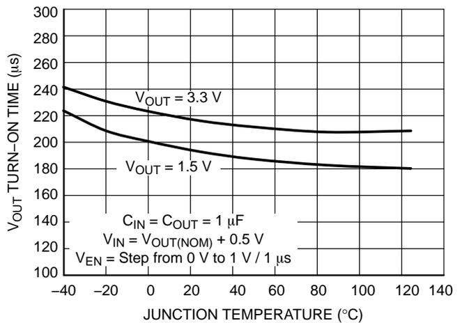
Figure 53. V<sub>OUT</sub> Turn-on Time vs. Temperature
