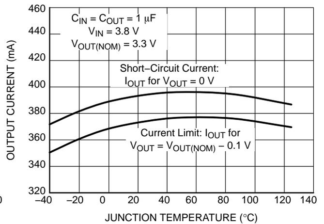
**Figure 29. Short-Circuit Limit vs. Temperature**
