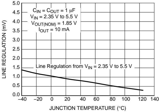
Figure 32. Line Regulation vs. Temperature
