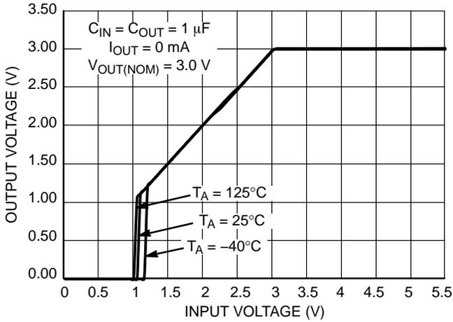
**Figure 14. Output Voltage vs. Input Voltage**
