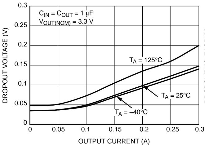
**Figure 22. Dropout Voltage vs. Output Current**
