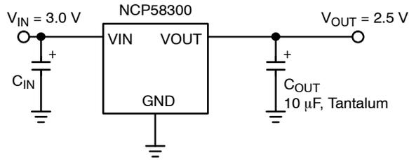
Figure 3. Fixed 2.5 Regulator in D<sup>2</sup>PAK-3 Package
