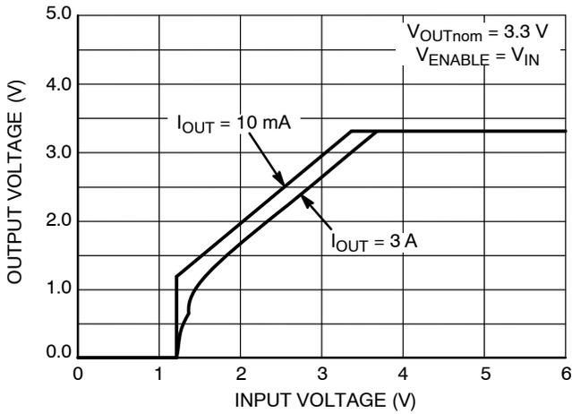
Figure 6. Dropout Characteristics
