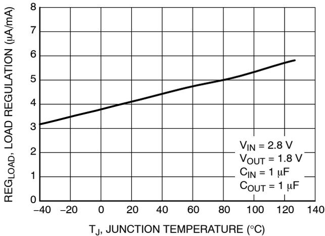
Figure 7. Load Regulation vs. Temperature -  $V_{OUT} = 1.8\text{ V}$
