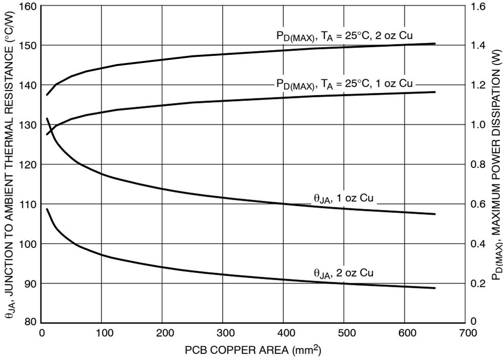
Figure 38.  $\theta_{JA}$  and  $P_{D(MAX)}$  vs. Copper Area (CSP4)
