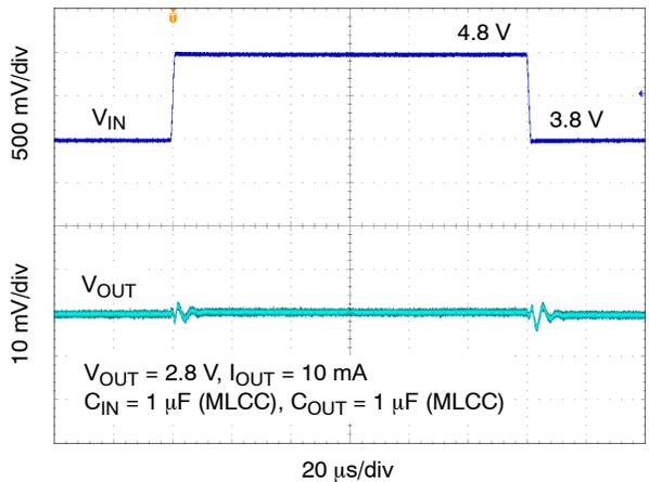
Figure 30. Line Transient Response –  $V_{OUT} = 2.8 \text{ V}$
