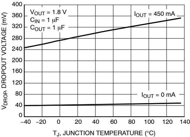
Figure 13. Dropout Voltage vs. Temperature -  $V_{OUT} = 1.8 V$
