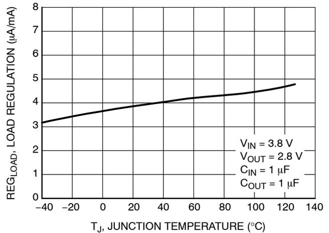
Figure 8. Load Regulation vs. Temperature -  $V_{OUT} = 2.8\text{ V}$
