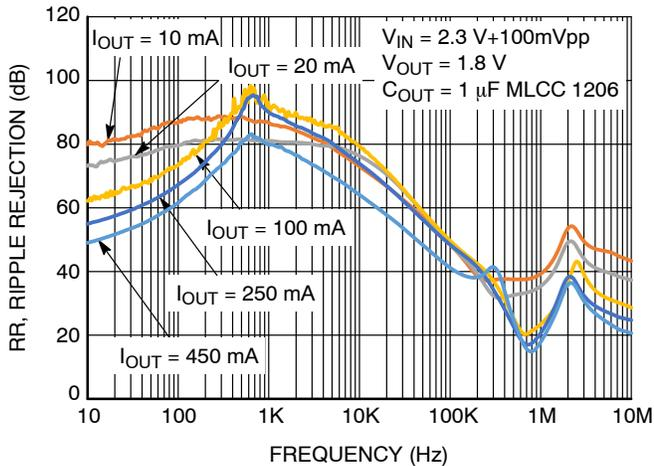
Figure 23. PSRR for Various Output Currents, V<sub>OUT</sub> = 1.8 V
