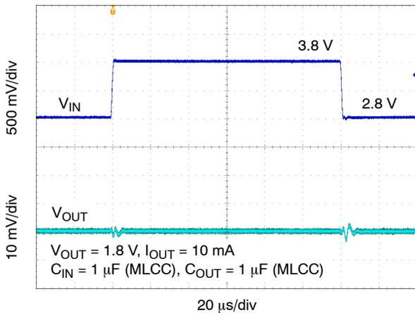
Figure 29. Line Transient Response –  $V_{OUT} = 1.8 \text{ V}$
