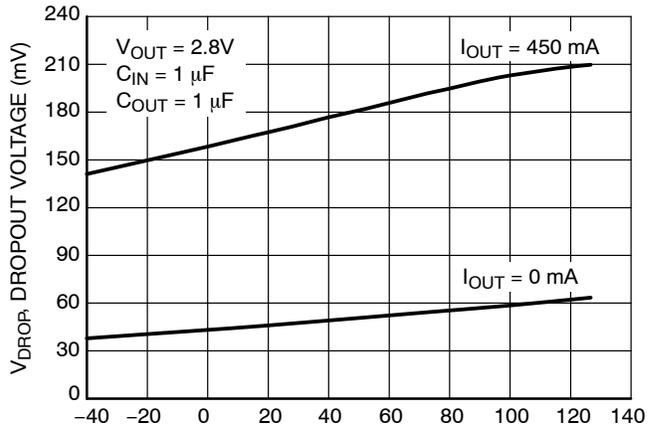
Figure 14. Dropout Voltage vs. Temperature -  $V_{OUT} = 2.8 V$
