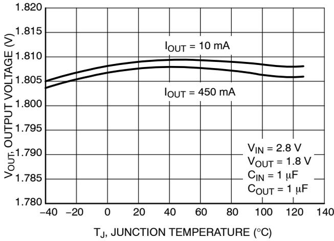
Figure 3. Output Voltage vs. Temperature -  $V_{OUT} = 1.8\text{ V}$
