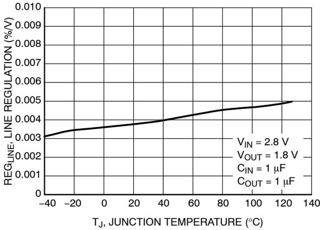
Figure 5. Line Regulation vs. Temperature -  $V_{OUT} = 1.8\text{ V}$
