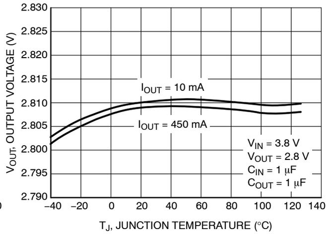
Figure 4. Output Voltage vs. Temperature -  $V_{OUT} = 2.8\text{ V}$
