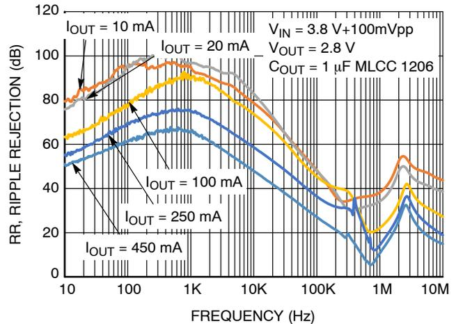
Figure 24. PSRR for Various Output Currents, V<sub>OUT</sub> = 2.8 V
