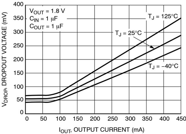
Figure 11. Dropout Voltage vs. Load Current -  $V_{OUT} = 1.8 V$
