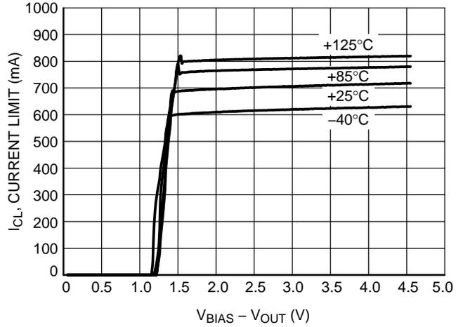
**Figure 11. Current Limit vs.  $(V_{BIAS} - V_{OUT})$**
