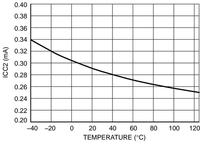
Figure 5. ICC2 @ V<sub>CC</sub> = 6.0 V, FB = Open vs. Temperature
