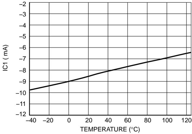
Figure 3. IC1 @ V<sub>CC</sub> = 8.0 V, FB = 1.5 V vs. Temperature
