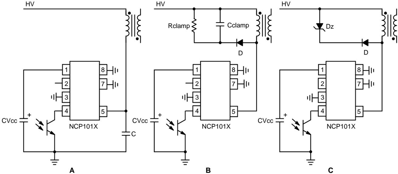
**Figure 29. Different Options to Clamp the Leakage Spike**
