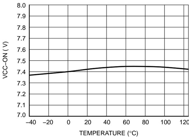
Figure 7. V<sub>CC</sub> ON, FB = 3.5 V vs. Temperature
