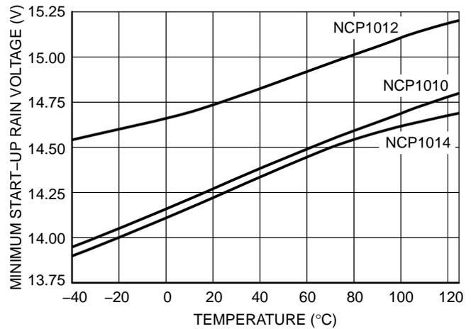
Figure 14. Minimum Start-up Drain Voltage vs. Temperature
