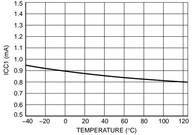
Figure 4. ICC1 @ V<sub>CC</sub> = 8.0 V, FB = 1.5 V vs. Temperature
