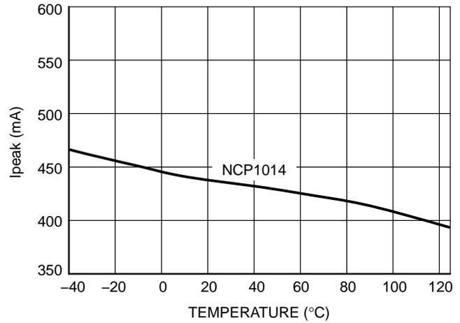
Figure 10. I<sub>peak-RR</sub>, V<sub>CC</sub> = 8.0 V, FB = 3.5 V vs. Temperature
