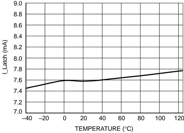
Figure 9. I<sub>Latch</sub>, FB = 1.5 V vs. Temperature
