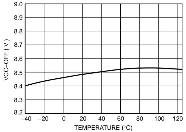
Figure 6. V<sub>CC</sub> OFF, FB = 1.5 V vs. Temperature
