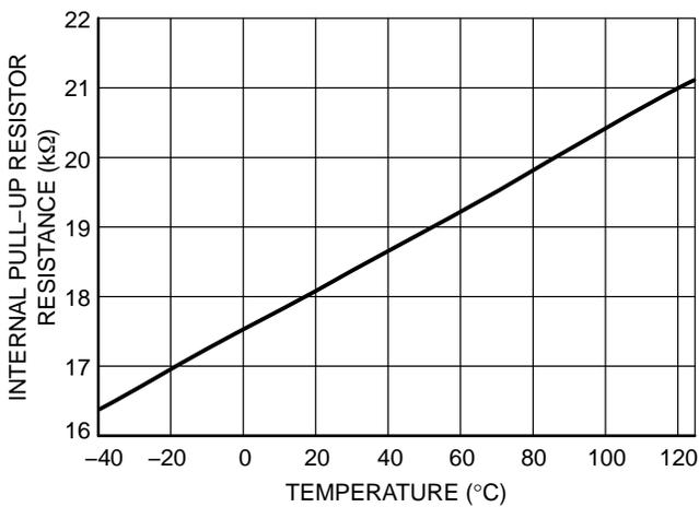
Figure 13. R<sub>up</sub> vs. Temperature
