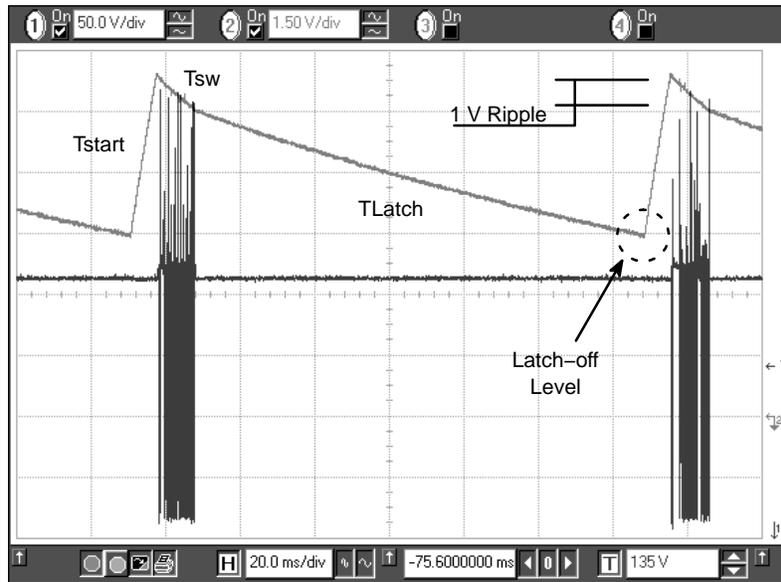
Figure 18. NCP101X Facing a Fault Condition (Vin = 150 Vdc)
