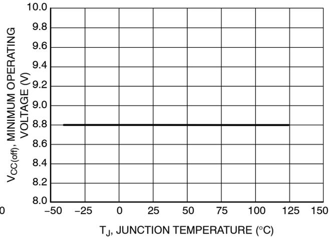
Figure 4. Minimum Operating Voltage vs. Junction Temperature
