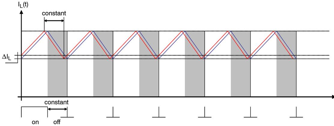
Figure 24. The Constant Off Time Technique is Immune to Sub-Harmonic Instabilities without Ramp Compensation
