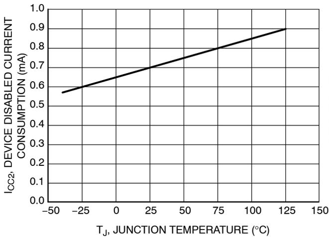
Figure 7. Device Disabled Current Consumption vs. Junction Temperature
