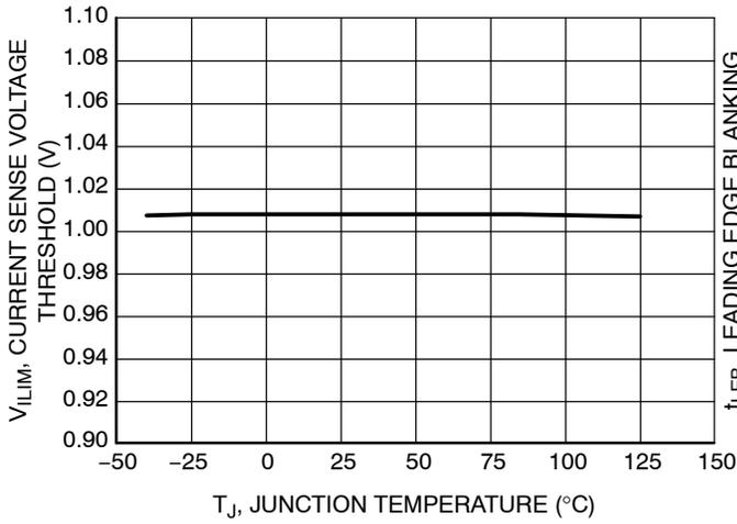
Figure 9. Current Sense Voltage Threshold vs. Junction Temperature
