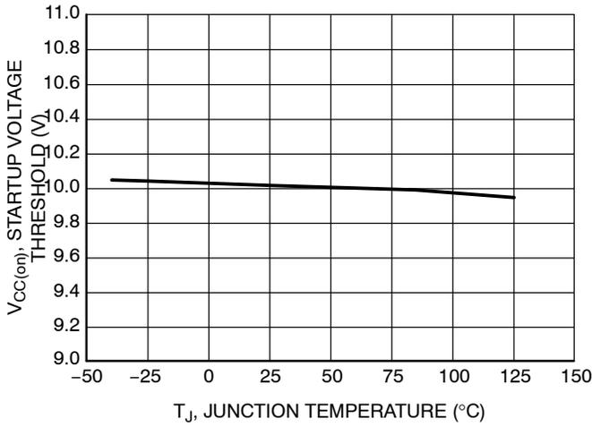
Figure 3. Startup Voltage Threshold vs. Junction Temperature
