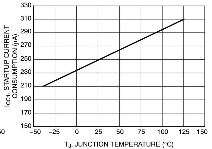
Figure 6. Startup Current Consumption vs. Junction Temperature
