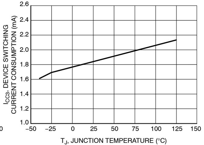
Figure 8. Device Switching Current Consumption vs. Junction Temperature
