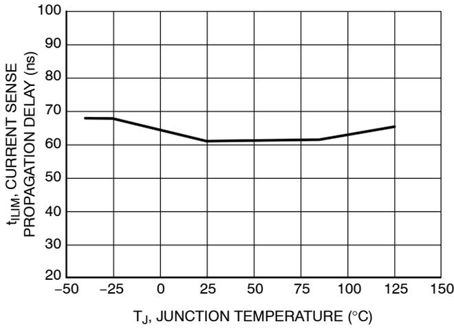
Figure 11. Current Sense Propagation Delay vs. Junction Temperature
