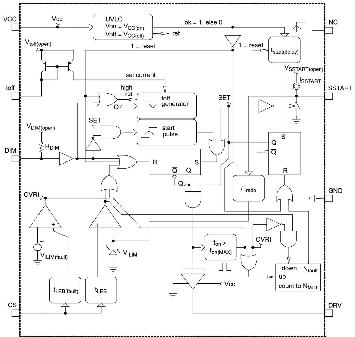
Figure 2. Internal Circuit Architecture
