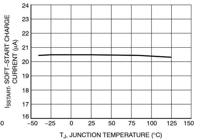
Figure 12. Soft-Start Charge Current vs. Junction Temperature
