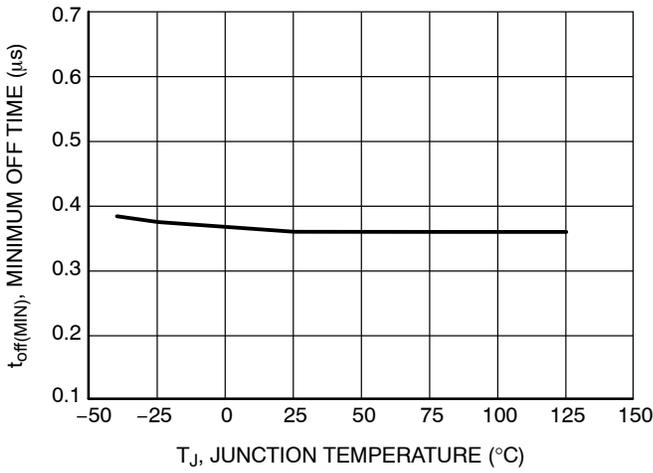
Figure 15. Minimum Off Time vs. Junction Temperature
