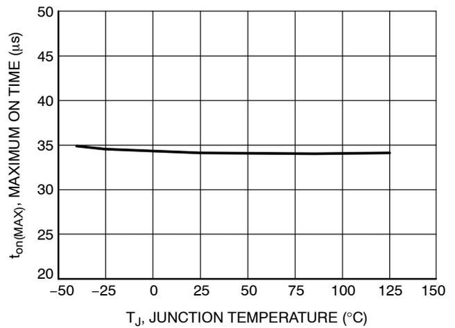
Figure 18. Maximum On Time vs. Junction Temperature
