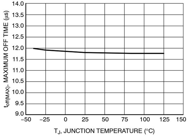
Figure 16. Maximum Off Time vs. Junction Temperature
