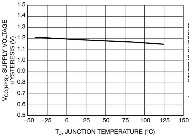
Figure 5. Supply Voltage Hysteresis vs. Junction Temperature
