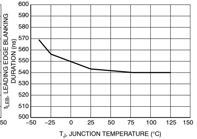
Figure 10. Leading Edge Blanking Duration vs. Junction Temperature
