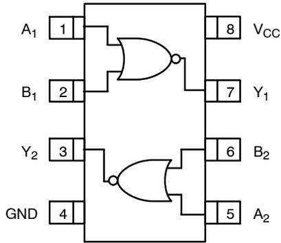
Figure 2. Pin Assignment for US8 (Top View)
