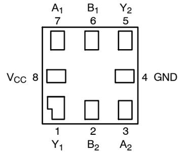
Figure 4. Pad Assignments for MicroPak (Top Through View)
