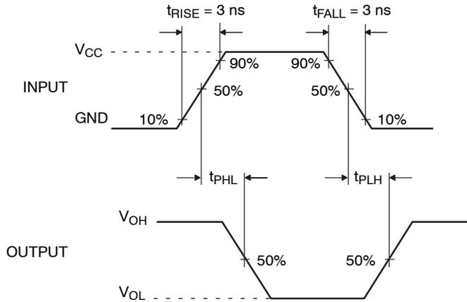
Figure 7. AC Waveforms
