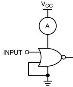
Input = AC Waveform; t<sub>r</sub> = t<sub>f</sub> = 1.8 ns;
