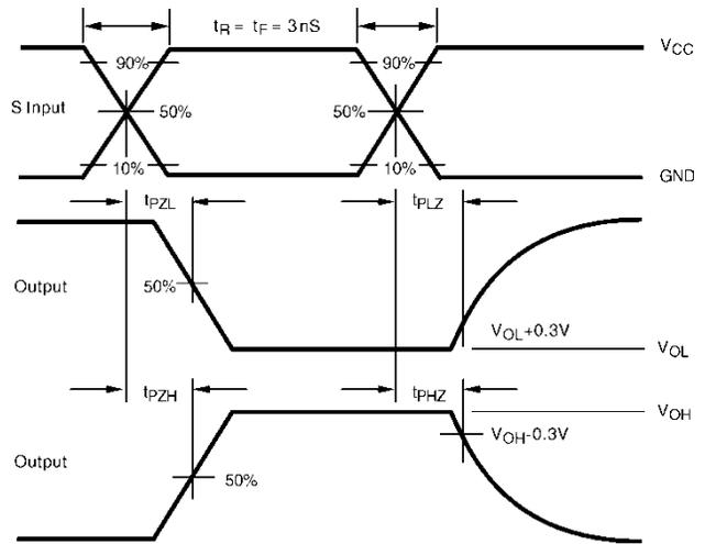
Figure 6. AC Waveforms
