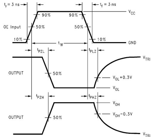
Figure 6. AC Waveforms
