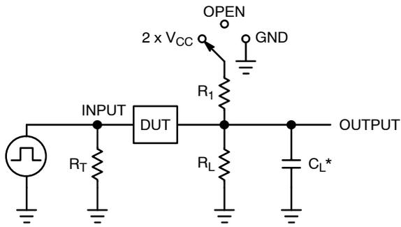
$C_L$  includes probe and jig capacitance
