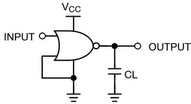
$C_L$  includes load and stray capacitance
