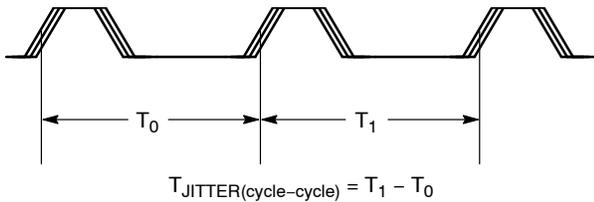
Figure 11. Cycle-to-Cycle Jitter
