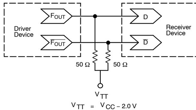
**Figure 19. Typical Termination for Output Driver and Device Evaluation**
