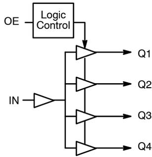
Figure 2. Block Diagram
