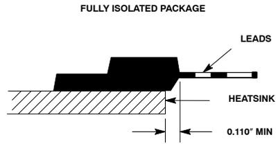
**Figure 3. Mounting Position**
