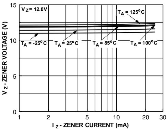
Figure 5. 12 Zener Voltage vs. Zener Temperature
