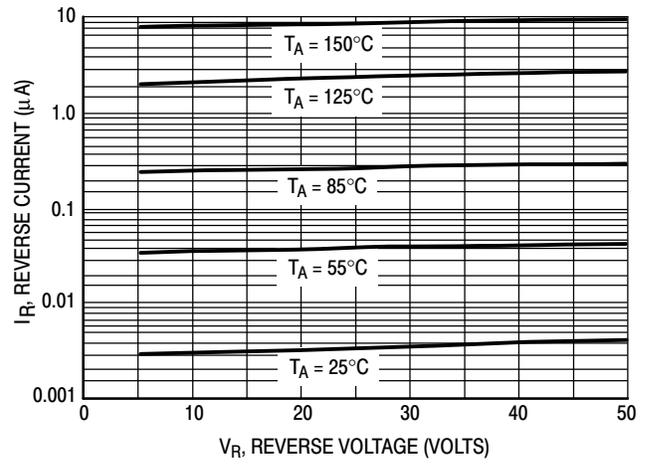
Figure 3. Leakage Current
