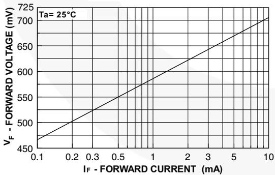
Figure 5. Forward Voltage vs. Forward Current
