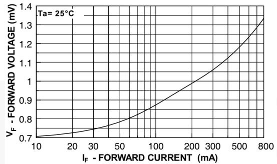
Figure 6. Forward Voltage vs. Forward Current
