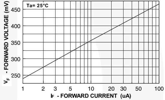
Figure 4. Forward Voltage vs. Forward Current
