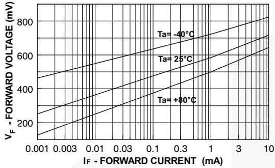
Figure 7. Forward Voltage vs. Ambient Temperature
