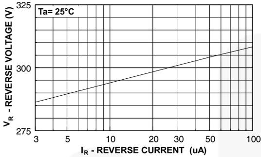
Figure 1. Reverse Voltage vs. Reverse Current
