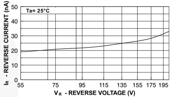
Figure 2. Reverse Current vs. Reverse Voltage
