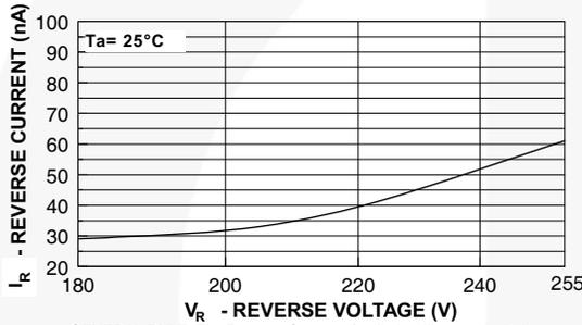
Figure 3. Reverse Current vs. Reverse Voltage
