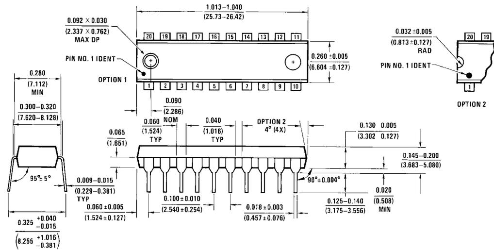
20-Lead Plastic Dual-In-Line Package (PDIP), JEDEC MS-001, 0.300" Wide
