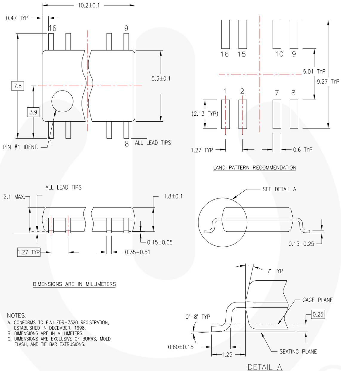
Figure 5. 16-Lead, Small Outline Package (SOP), EIAJ TYPE II, 5.3mm Wide
