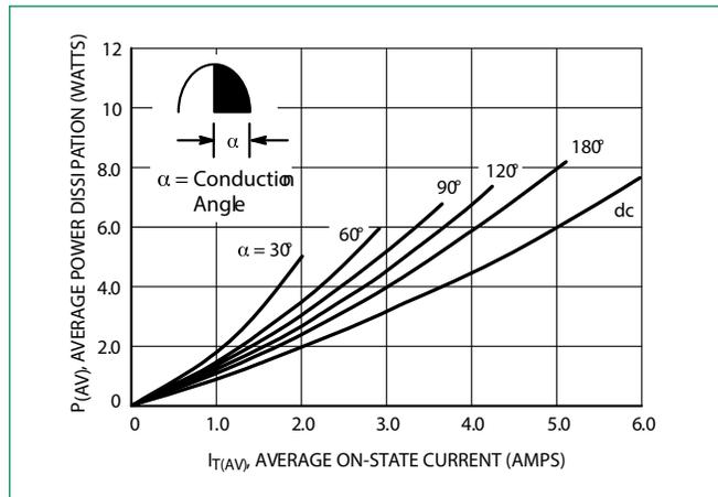
**Figure 3. On-State Characteristics**
