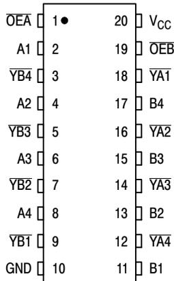
Figure 1. Pin Assignment
