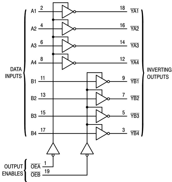
Figure 1. LOGIC DIAGRAM
