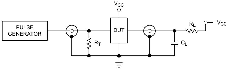
$C_L = 50 \text{ pF}$  equivalent (Includes jig and probe capacitance)
