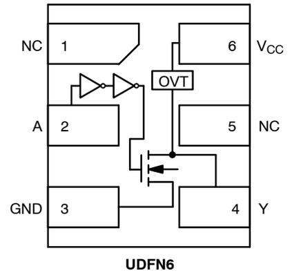
Figure 2. Pinout (Top View)
