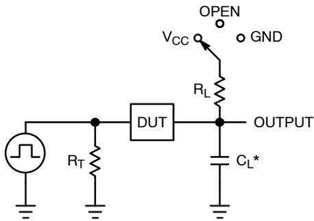
$C_L$  includes probe and jig capacitance
