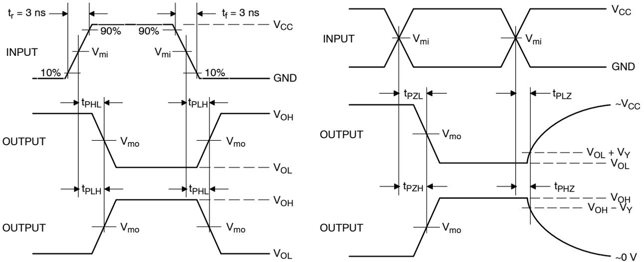
**Figure 4. Switching Waveforms**
