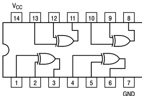
Figure 1. Pinout: 14-Lead Packages Conductors (Top View)
