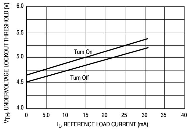
**Figure 10. Undervoltage Lockout Thresholds versus Reference Load Current**
