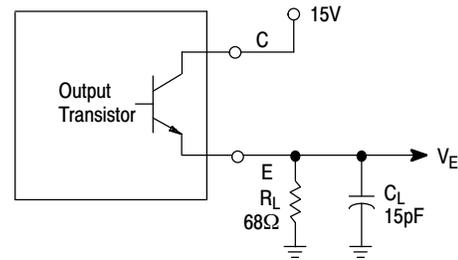
Figure 14. Emitter-Follower Configuration and Waveform
