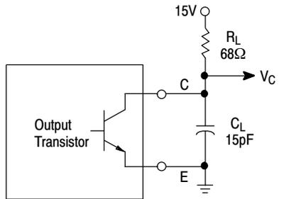
Figure 13. Common-Emitter Configuration and Waveform
