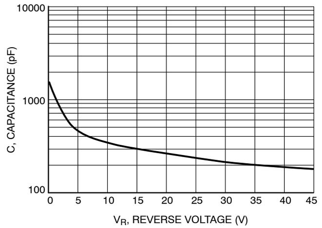
Figure 7. Typical Capacitance
