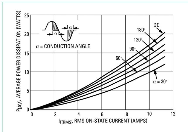
Figure 3. On-State Characteristics
