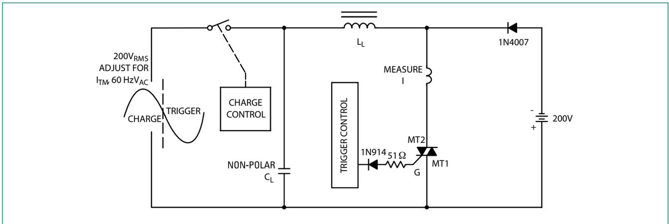
Note: Component values are for verification of rated (di/dt)<sub>c</sub>. See AN1048 for additional information
