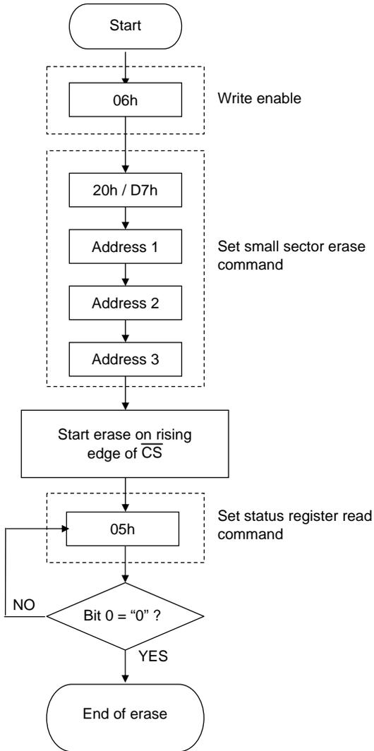
\* Automatically placed in write disabled state at the end of the erase
