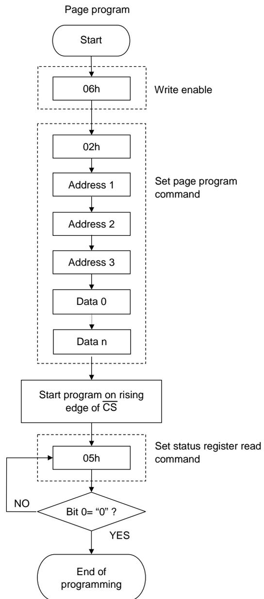
\* Automatically placed in write disabled state at the end of the programming operation.
