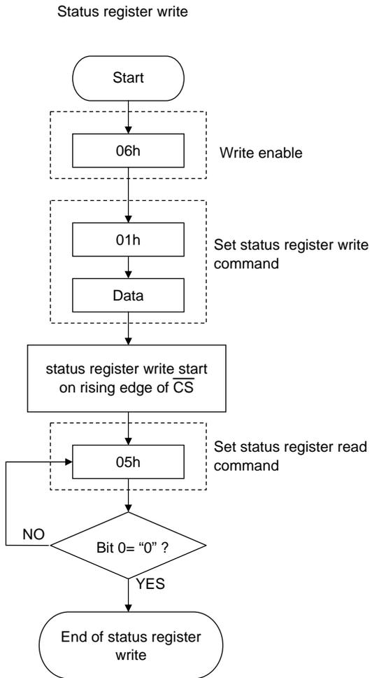
\* Automatically placed in write disabled state at the end of the status register write
