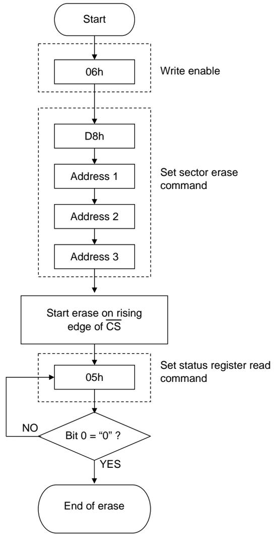
\* Automatically placed in write disabled state at the end of the erase
