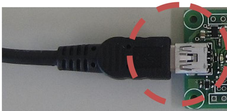
Figure 5. Connection via USB-Mini Cable
