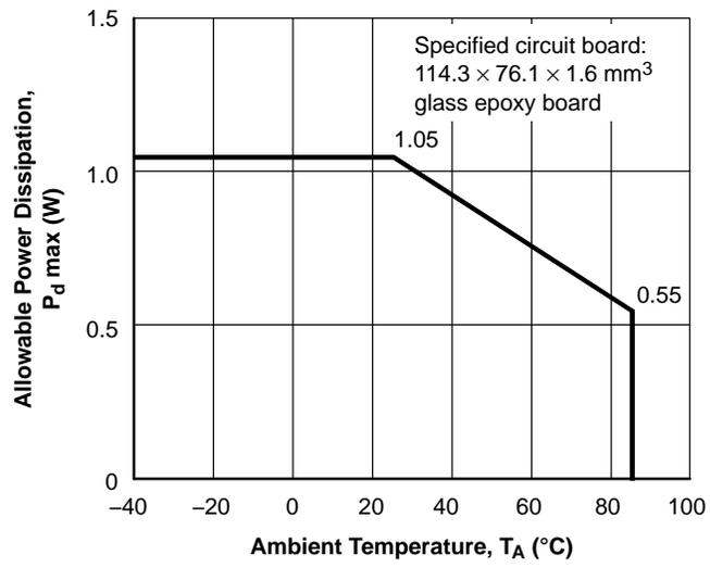
Figure 1. P<sub>d</sub> max – T<sub>A</sub>
