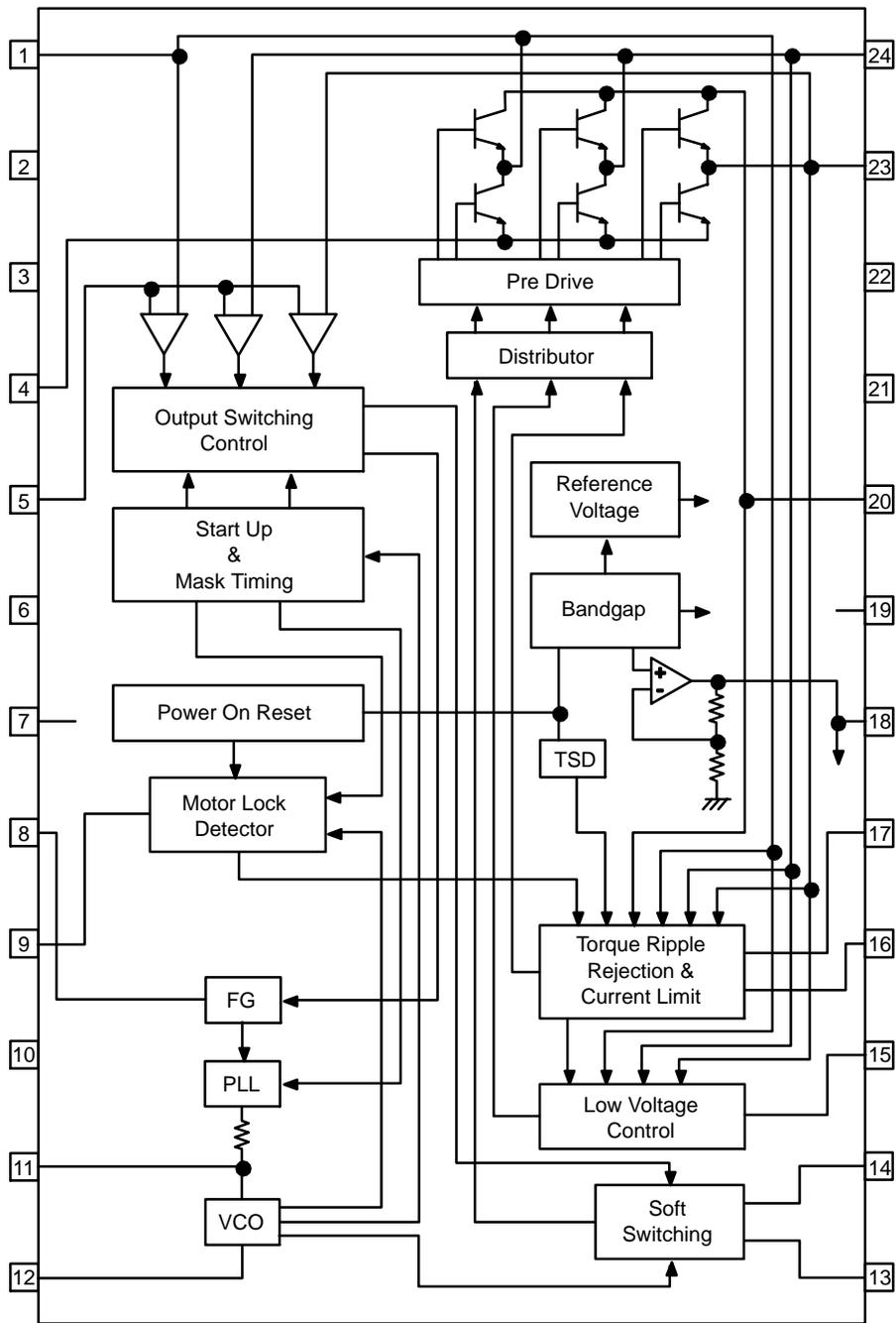
Figure 2. Block Diagram
