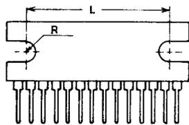
3. The screw to be used must have a head equivalent to the one of truss machine screw or binder machine screw defined by JIS. Washers must be also used to protect the IC case.
