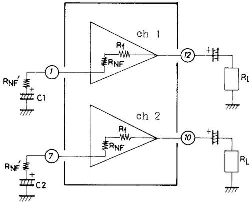
$R_{NF}=50\Omega$  (typ),  $R_f=20k\Omega$  (typ)
