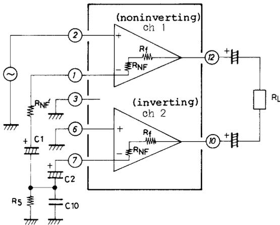
$$VG=20\log \frac{R_f}{\frac{R_{NF}+R_{NF}'}{2}} \text{ (dB)}$$
