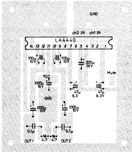
Sample printed circuit pattern for dual mode (Cu-foiled area) 60 x 70 mm<sup>2</sup>
