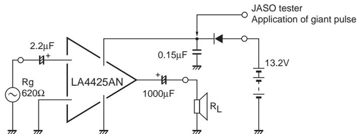
The over-voltage protector ( $V_{CCX} \approx 21.5V$ ) inside the IC is used to cut all bias routes and reverse bias between B-E of output stage elements, in order to increase the power line's capability of handling positive surge. This means, of course, that a  $V_{CES}$  ( $V_{CBO}$ ) type output stage element is used instead of the  $V_{CEO}$  ( $V_{CER}$ ) type.
