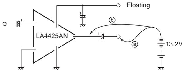
The power pin is in a floating state when a power capacitor is connected, so if +V<sub>CC</sub> touches output lines (a) and (b), the upper power transistor inside the IC will be damaged.
