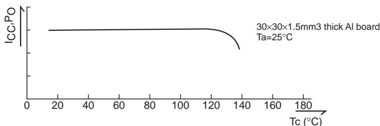
T.S.D is capable of starting operation at T<sub>c</sub> 120 to 130°C. When this is converted to junction temperature (T<sub>j</sub>) according to the formula below.
