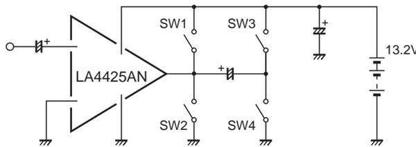
Our company's recommended printed circuit board: Apply  $V_{CC}=13.2V$  using a  $30 \times 30 \times 1.5\text{mm}^3$  thick aluminum board. The IC will be protected from the DC/AC shorting of switches 1 to 4 above. However, be careful not to damage the IC by turning  $V_{CC}$  "ON" when DC short (SW 1 or SW 2) is on.
