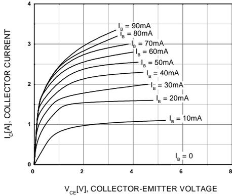
Figure 1. Static Characteristic
