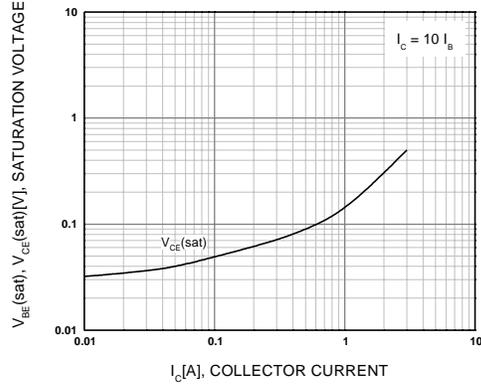
Figure 4. Collector-Emitter Saturation Voltage vs Collector Current
