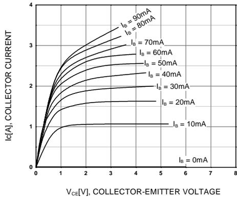
Figure 1. Static Characteristic
